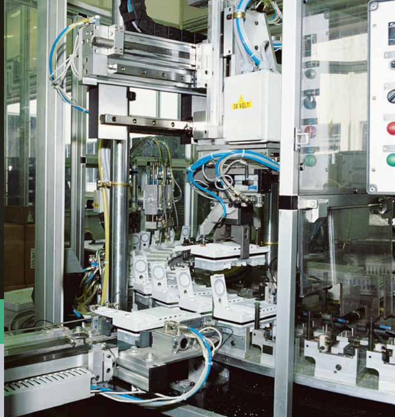
Dishwasher dosing units are produced fully automatically. After the injection moulding process, assembly of the finished components takes place on the assembly corridor.
