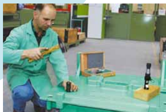
Hardness tests using the shearing pin method in production control
