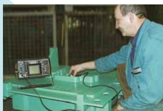
ARBURG leaves nothing to chance: ultrasound inspection to identify internal faults
